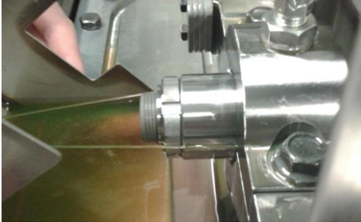
*Figure 50. Oil spewing out of bearing*
