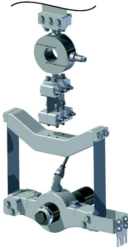
*Figure 36. How to remove bearing housing assembly*
