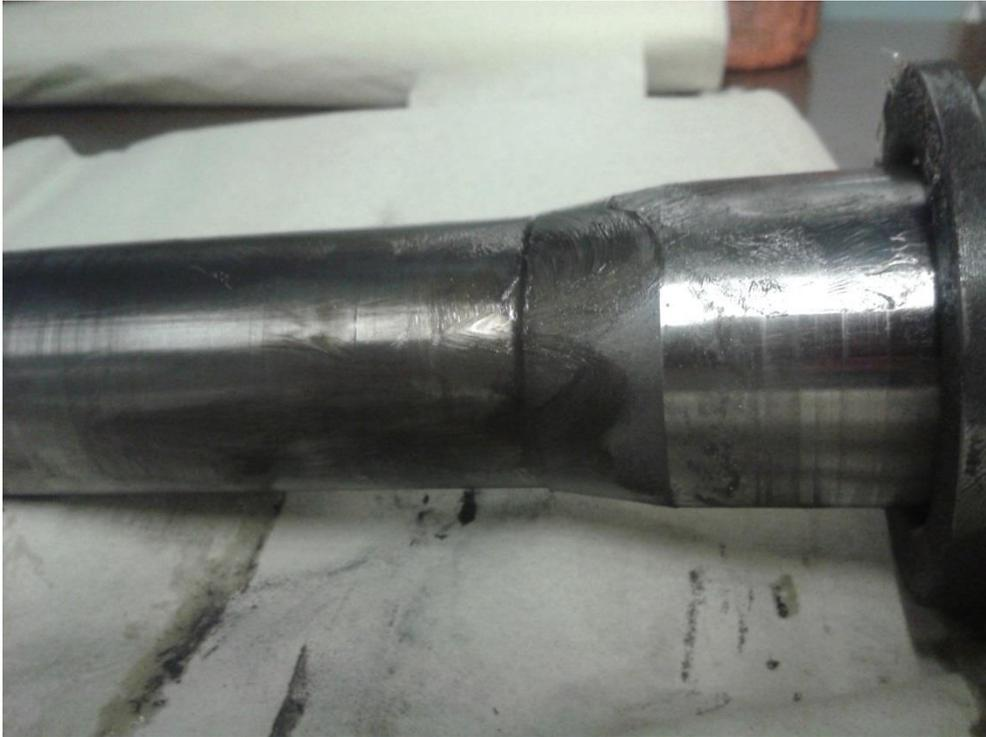
*Figure 72. View of destroyed inner radius at chamfer*
