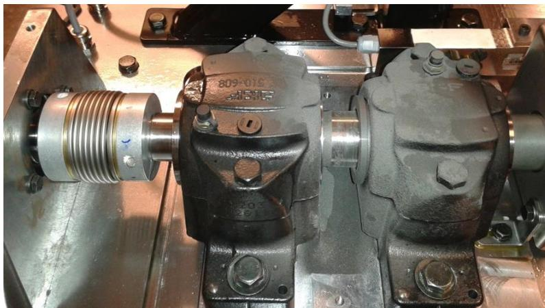
Figure 69. Overview of damaged support bearing housing
