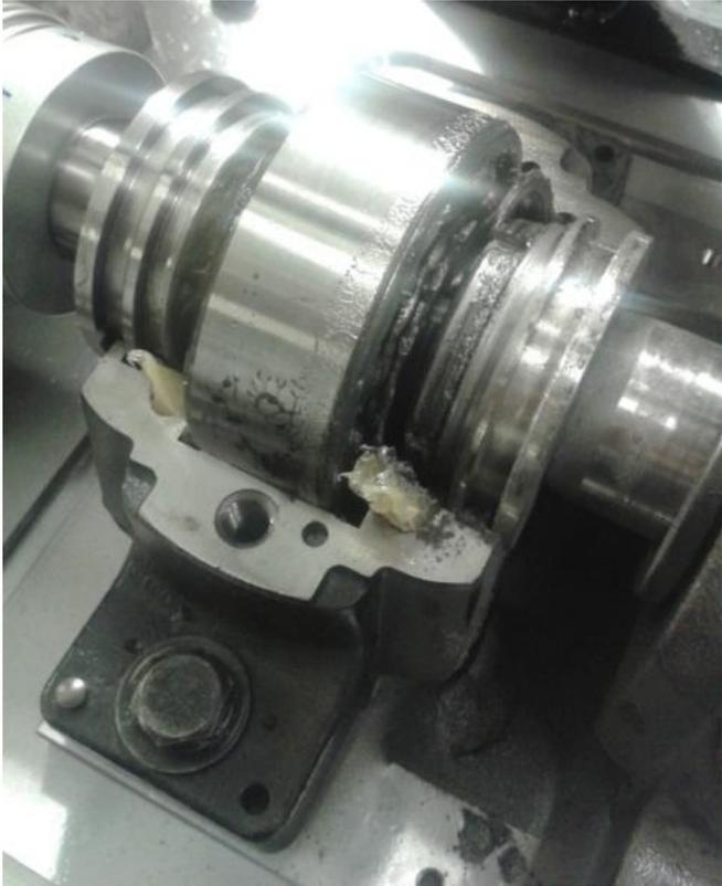
*Figure 70. View of contaminated bearing and damaged bearing housing*
