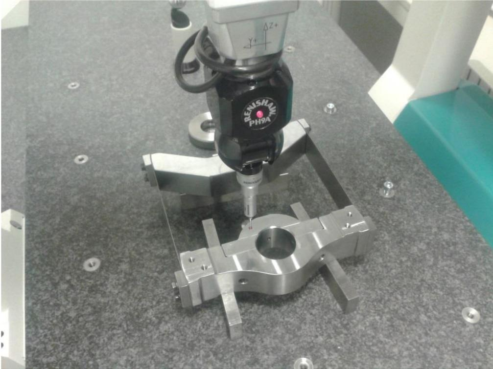
*Figure 7. CMM measuring flatness of the bearing housing*
