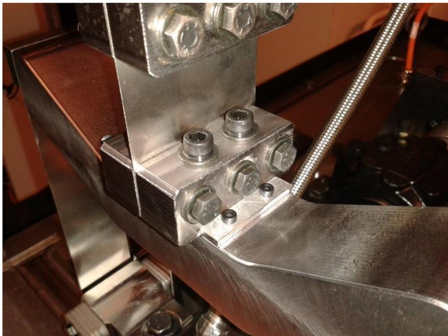
*Figure 37. Positional guide on the yoke*
