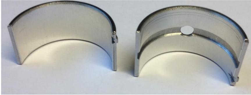
Figure 3. Steel bearing shells with aluminium liner from a Scania DL5 balance shaft module
