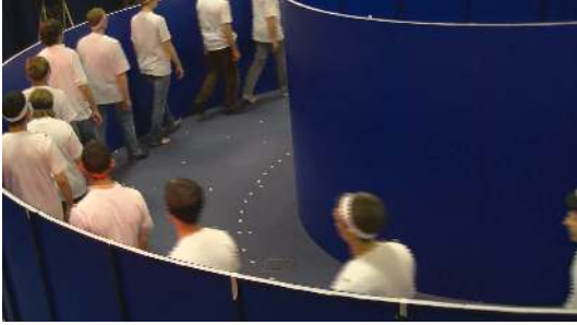
Figure 1: Experiments on 1-D traffic: participants were asked to walk without overtaking each other. At the microscopic scale, we observe how humans adapt their motion to follow someone. At the macroscopic scale, we observe the emergence of stop-and-go waves from such interactions: the trough of such a wave is visible on picture's leftest part.
