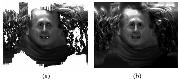
Figure 2: (a) Texture data of “George” with void points displayed in white and (b) texture image interpolated using relaxation method.
