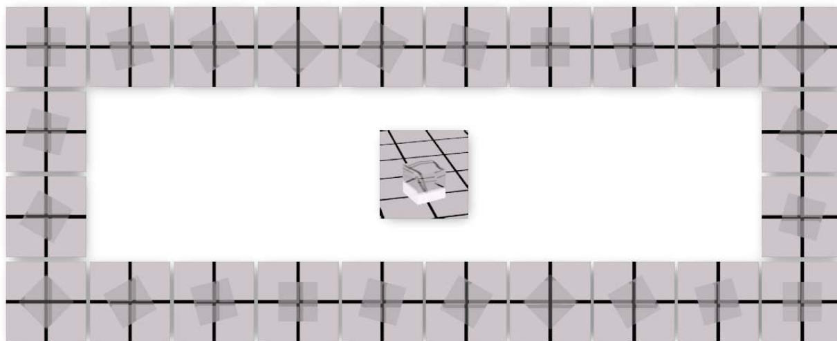
Fig. 7. Orientation-dependency of birefringence. The rotation angle of the cube was increased at steps of 15^\circ from image to image. n_o = 1.3 and n_e = 1.5 . The optical axis was originally (0.577, 0.577, 0.577) .
