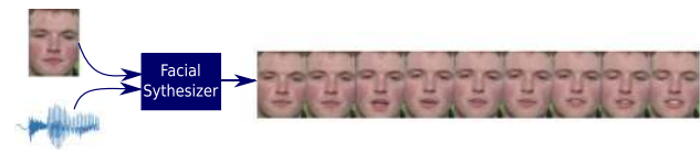
Fig. 1 The proposed end-to-end face synthesis model, capable of producing realistic sequences of faces using one still image and an audio track containing speech. The generated sequences exhibit smoothness and natural expressions such as blinks and frowns
