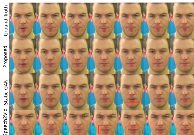
Fig. 18 Example of consecutive frames showcasing the failure of static methods to produce a coherent motion. During silent periods static approaches exhibit jittery motion in the mouth
