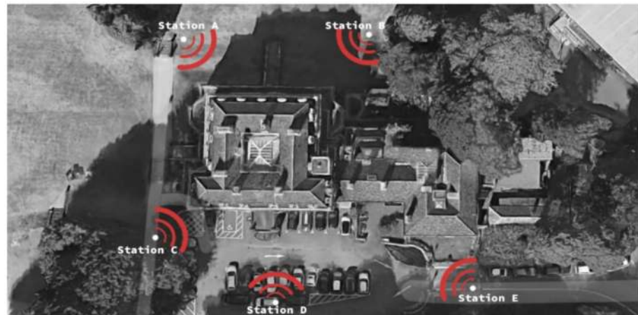
Figure 5. External scanning point placement on the Headington Hill Building site.
