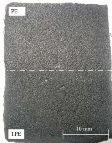
Fig. 8 Top-view image of PE and TPE multi-material part
