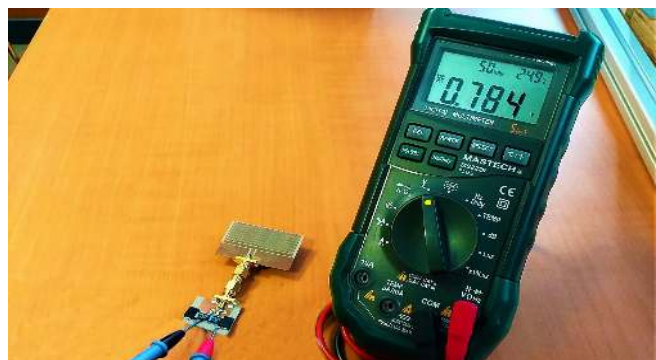
Figure 23. Measured output DC voltage using multimeter.
