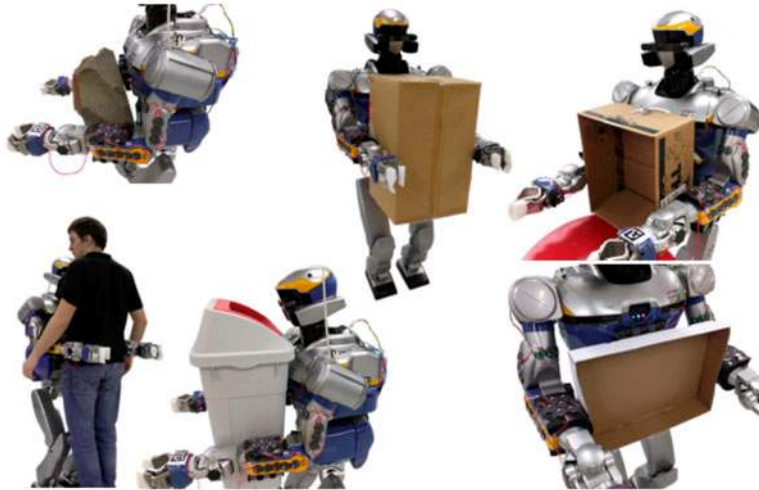
Figure 17. A position controlled HRP-2 humanoid, holding unknown objects with the whole-body, as result of a multi-modal tactile grasping sequence.
