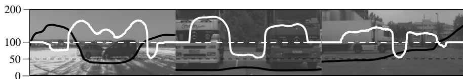
Fig. 5. Obstacle detection with distance histogram (black, scale on the left) and hypotheses verification (white, logarithmic scale, obstacle verified if above dashed line). The images show, that robust obstacle detection and verification is reached.
