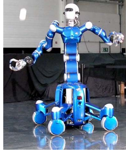
Fig. 8. DLR’s Rollin’ Justin catching a ball. For robust catching, the necessary accuracy is about 2cm in space and 5ms in time.
