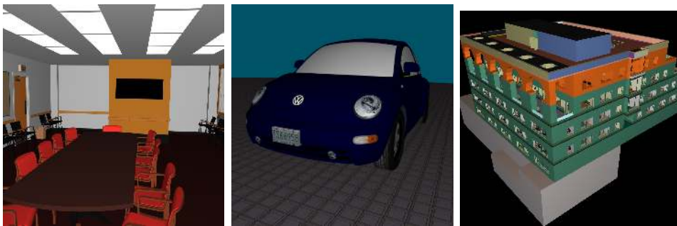
Figure 4.17: A small set of triangular example scenes for illustrating traversal statistics in the context of ray bundles. The scene complexity varies from left to right: 280K (Conference), 680K (VW Beetle), 2.16M (Soda Hall) triangles. All test scenes are rendered at a resolution of 1024 \times 1024 , using only primary rays.
