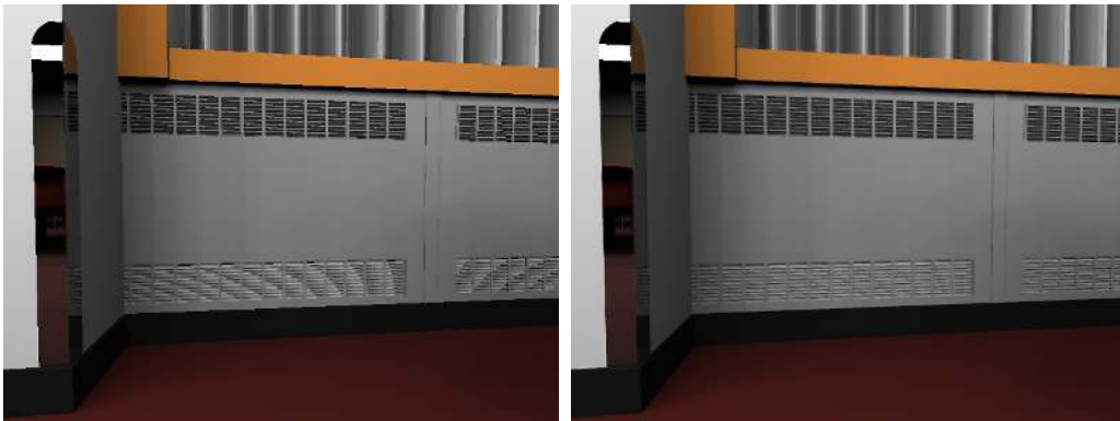
Figure 9.5: Left: Casting a single primary ray per pixel exhibits aliasing artifacts for small geometric details. Right: Casting four primary rays per pixel with interleaved shadow ray generation. As the number of shadow rays is constant, performance decreases only from 4 fps to 3.2 fps while providing better image quality through anti-aliased rendering.
