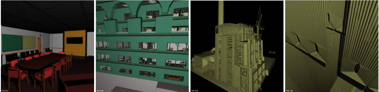
Figure 1: The CONFERENCE, SODA HALL, POWER PLANT from outside, and POWER PLANT furnace scenes. Using our new BVH-based GPU ray tracer, we render them at 6.1, 5.7, 2.9, and 1.9 fps, respectively, at a resolution of 1024 \times 1024 with shading and shadows from a single point light source.
