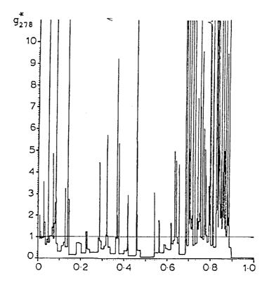
Figure 9 Medians of spline recalibrated predictions of  $T_{106}$  through  $T_{278}$ , JM and LV models, Musa SS3 data. Note closeness to results in Figure 7 for joined-up recalibration.
