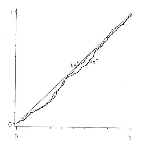
Figure 7 Medians of (joined-up) recalibrated predictions of  $T_{106}$  through  $T_{278}$ , JM and LV models, Musa SS3 data [17].
