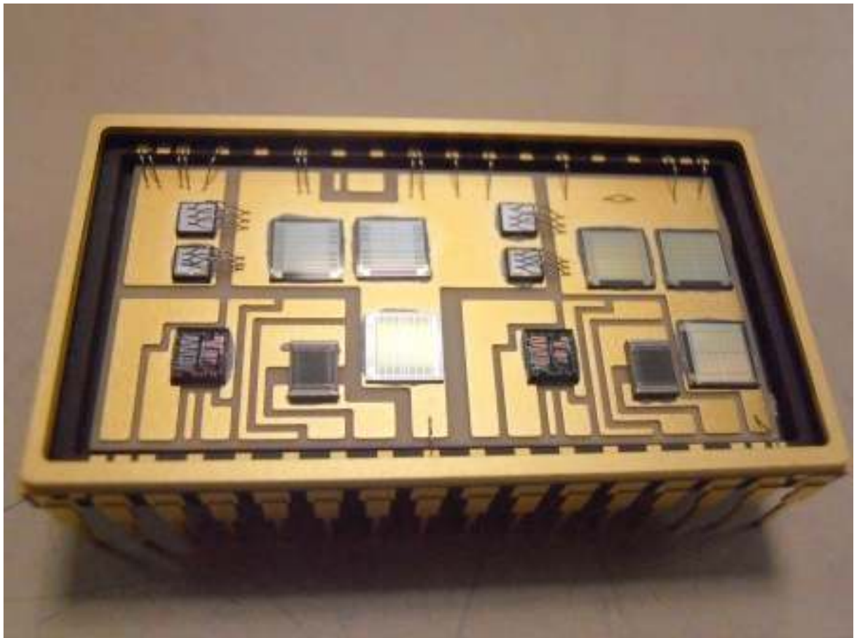
Image of a bridge leg assembly with SiC drivers, transistors and passive devices. The module is packaged in a 32-pin hermetic dual in-line (DIL) ceramic package measuring about 40mm x 23mm.
