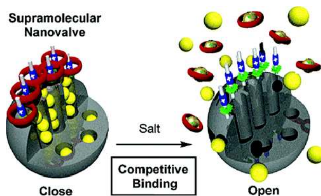
Figure 9. Graphical representation of operating supramolecular nanovalves from DB24C8/dialkylammonium-tethered porous silica particle MSNs. Reproduced with permission from [94]. Copyright American Chemical Society, 2006.
