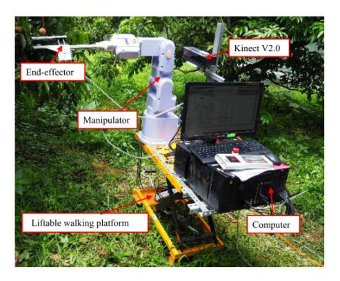
Figure 18. Robotic system for lychee harvesting [26].
