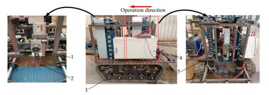
**Figure 12.** 1. Transplanting robot arm; 2. Transplanting position; 3. Crawler chassis; 4. Control box; 5. Filling robot arm [65].
