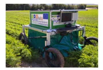
**Figure 10.** A remotely-driven RobHortic operating in a carrot field, showing the external appearance of the robot [52].
