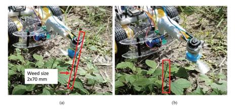
**Figure 17.** (Color online) Weeds (**a**) before cutting with a cutter blade and (**b**) after cutting with a cutter blade [86].
