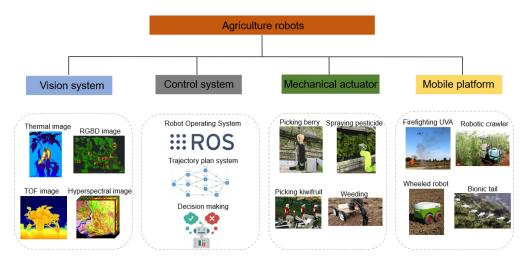
Figure 5. Implications of robotic components [14,19,20,26–30].
