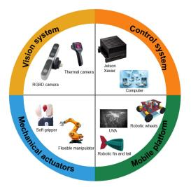
Figure 4. Components of agricultural robots [18,19].
