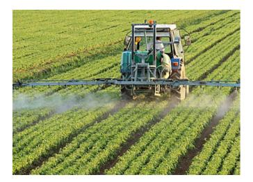
Figure 9. Tractor-mounted boom sprayer [50].
