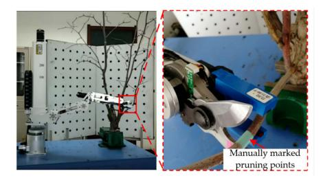
Figure 16. The pruning test [85].
