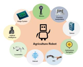
Figure 2. Core technologies involved in agricultural robotic applications.
