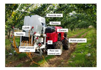
Figure 14. Intelligent spraying system [72].
