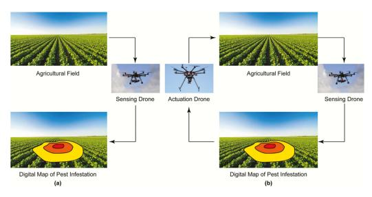
**Figure 8.** (a) State-of-the-art open-loop remote sensing paradigm and (b) closed-loop IPM paradigm envisioned in [44]. Sensing drones can be used to detect pest hotspots, while actuation drones can be used for precision distribution of solutions.
