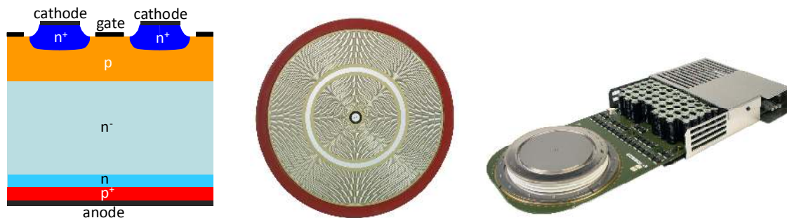
Fig. 1: IGCT device. Left: schematic cross section of Asymmetric IGCT. Middle: top view of 91mm IGCT wafer. Right: the IGCT wafer in a hermetic package and with its integrated gate unit.
