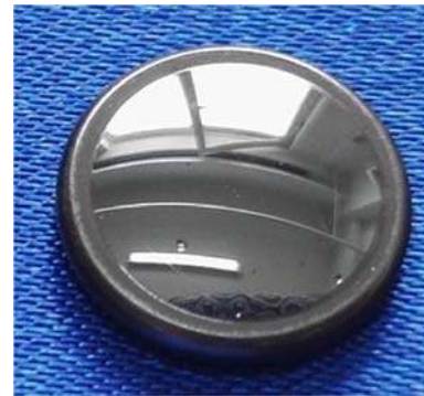
Fig. 35 Photograph of chalcogenide glass lens fabricated through GMP
