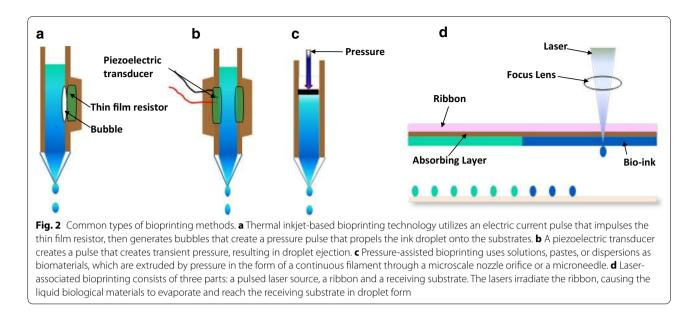
technology, the piezoelectric method does not use heat and does not cause orifice clogging, allowing droplets to remain directional with regular and equal size [25, 26]. However, piezoelectric technology can cause damage to the cell membrane and cell lysis if used too frequently [27]. Greater than 90 % viability has been reported for piezoelectrically deposited mammalian cells, including human osteoblasts, fibroblasts, and bovine chondrocytes [26].
