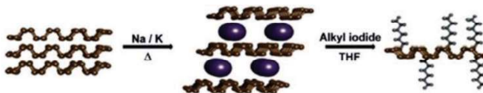
Figure 13. Reaction of BP intercalation compounds with alkyl halides through nucleophilic substitution. Reproduced with permission. [189] Copyright 2019, John Wiley and Sons.
