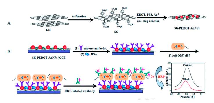
**Figure 4.** Principle of the sandwich assay. **(A)** Synthesis of sulfonated graphene (SG-PEDOT-AuNPs) composites and Poly-(3,4- 444 ethylenedioxythiophene) (PEDOT) in a single step reaction; **(B)** Schematic representation of electrochemical reaction where antibody was bound on the surface of glassy carbon electrode and detection of target by change in current. Adapted with permission from Ref. [82]. Copyright 2020, Elsevier.
