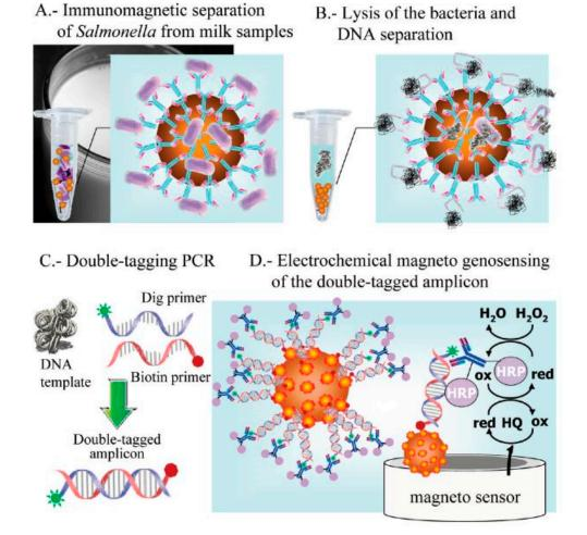
**Figure 5.** Electrochemical genosensing using immunomagnetic separation (IMS)/double-tagging PCR/m-GEC technique. (**A**) Separation of *Salmonella* contamination using Immunochromatographic separation in milk samples; (**B**) Bacterial lysis and separation of the nuclei acid; (**C**) Double-tagging of the nucleic acids; (**D**) Electrochemical genosensing (GEC) of double-tagged amplicon or the nucleic acid. Adapted with permission from Ref. [84]. Copyright 2009, American Chemical Society.
