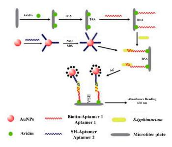
**Figure 2.** Detection of *Salmonella typhimurium* via attachment of avidin and AuNPs for recognition of biotinylated aptamer 1 and SH-aptamer 2, respectively. Adapted with permission from Ref. [22]. Copyright 2014, Elsevier.
