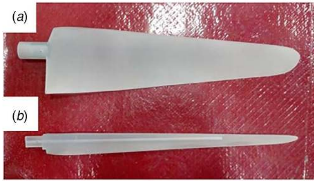
Fig. 11 Wave basin testing of floating offshore wind turbines: (a) and (b) thrust-scaled blade versus geometrically scaled blade [130], (c) thrust coefficient for a thrust-scaled 5 MW wind turbine [136], and (d) hybrid test model using multi-fan [137] (an example of a hybrid test model using motor and wire actuators [138] can be seen in Fig. 12)
