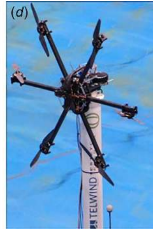
Fig. 11 Wave basin testing of floating offshore wind turbines: (a) and (b) thrust-scaled blade versus geometrically scaled blade [130], (c) thrust coefficient for a thrust-scaled 5 MW wind turbine [136], and (d) hybrid test model using multi-fan [137] (an example of a hybrid test model using motor and wire actuators [138] can be seen in Fig. 12)
