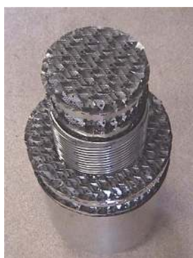
Fig. 6 The structure of the shell and tube installed in the HIDiC
