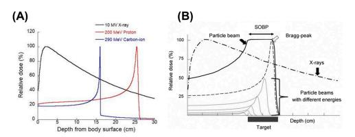
**Figure 1.** (**A**) Depth-dose distributions of clinical X-ray, proton, and carbon-ion beams, and (**B**) the spread-out Bragg peak (SOBP). Reproduced from [5], with permission from Elsevier, Copyright 2021.
