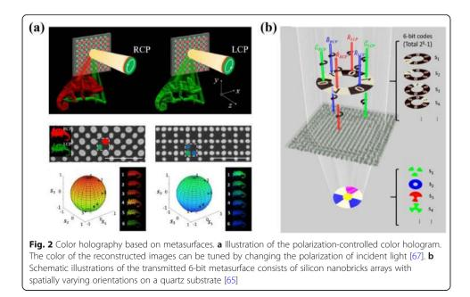
designed observed plane. Other color holography scheme has been achieved by utilizing multiple polarization channels. A non-interleaved  $TiO_2$  metasurface hologram is demonstrated with capabilities of encoding three distinct phase profiles in different polarization channels. Combining three polarization channels with three primary color channels, a full-color hologram with nearly no crosstalk is realized [68].
