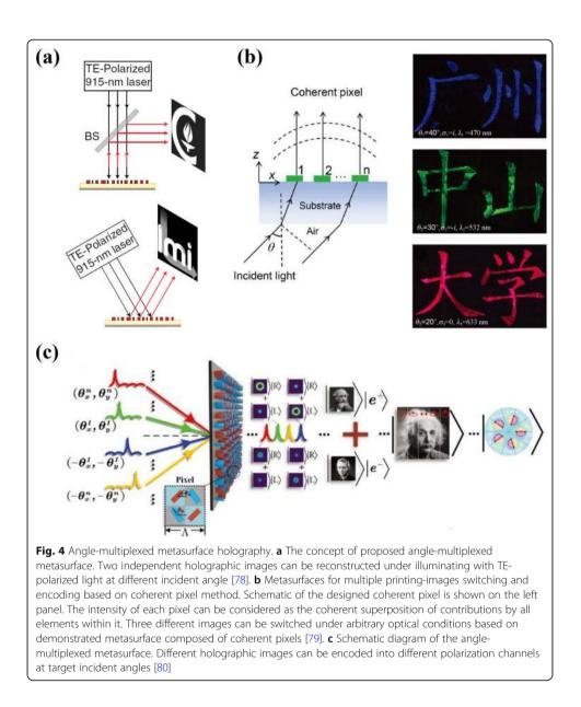
output light by combining the coherent pixel method together with geometric phase principle, as shown in Fig. 4c. The proposed method provides a facile route to obtain multichannel, angle-multiplexed and arbitrary spatially varying polarization fields and can be utilized to achieve novel applications such as full Poincaré beams generation, dual-way switching print images, vectorial printing-images, and optical polarization knot profiles generation.
