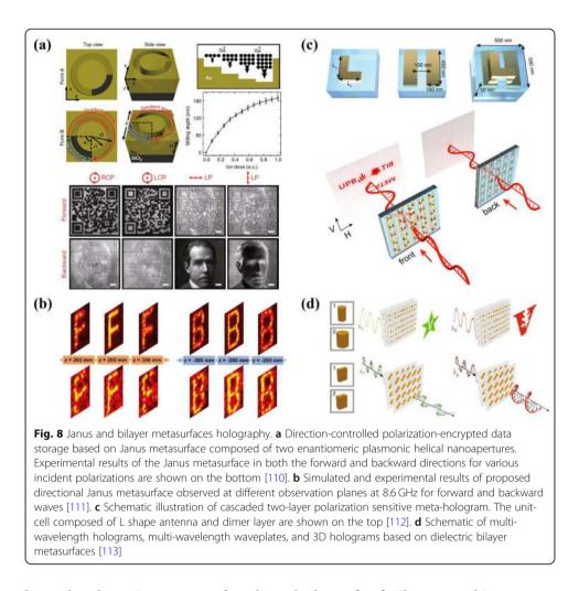
be used to design Janus metasurfaces by multiplexing [111]. The proposed Janus metasurfaces can break out-of-plane symmetry and enable different functions for opposite propagation directions and realized functionalities including one-way anomalous refraction, one-way focusing, asymmetric focusing, and direction-controlled holograms as shown in Fig. 8b.
