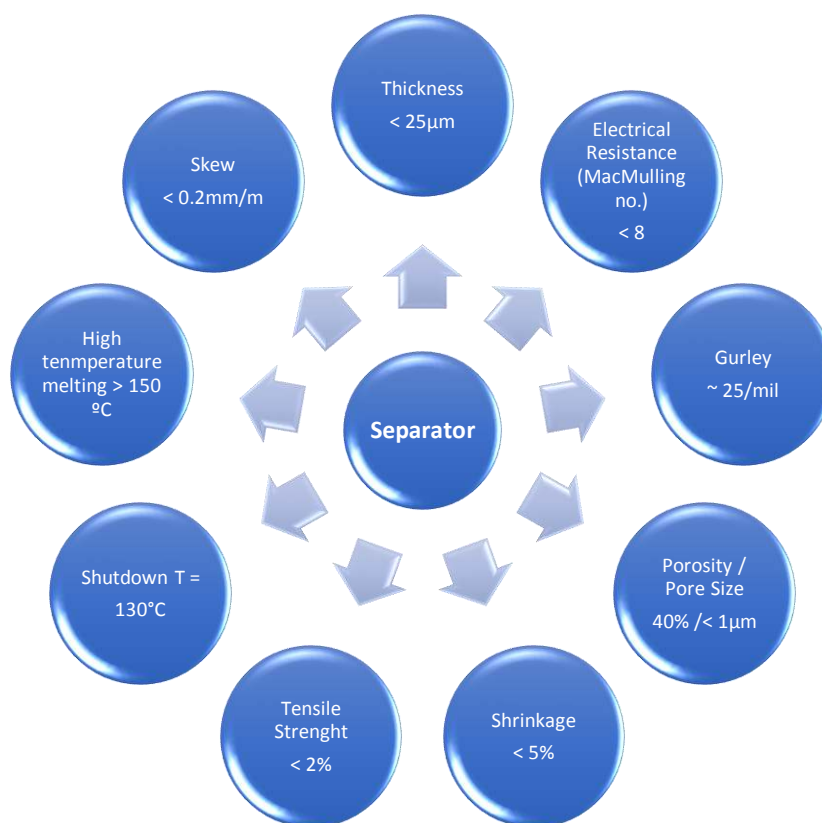
Figure 2 – Ideal values for the main requirements of a separator membrane.
