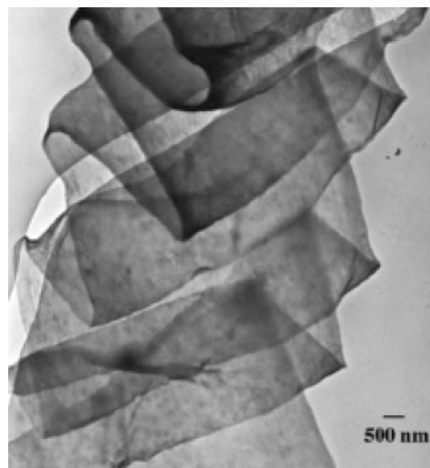
28 Micrograph (TEM) of ribbon shaped nanofibre. Reprinted with permission from Ref. 74, © 2002, Elsevier Science
