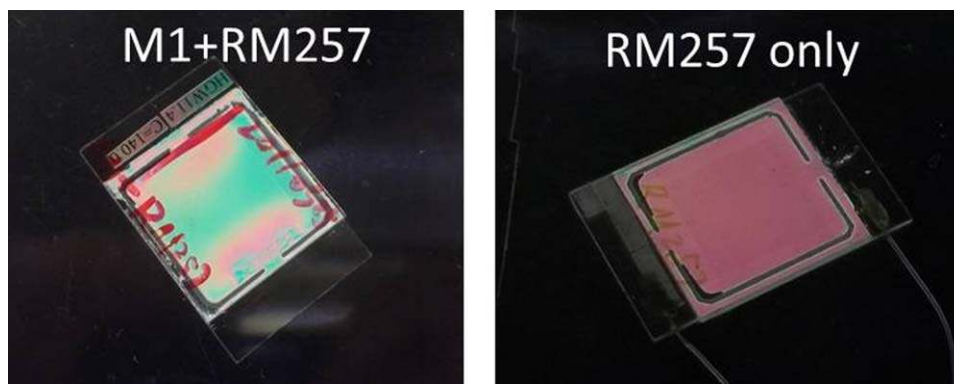
FIGURE 7 Photographs of two PNLCs containing different types of monomers.
