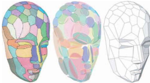
Fig. 18. Error-driven remeshing: Through repeated error-driven partitioning (left), a set of geometric proxies (represented as ellipses, center) is optimized. These proxies are then used to construct an approximating polygonal mesh (right). Figure reproduced from [16].
