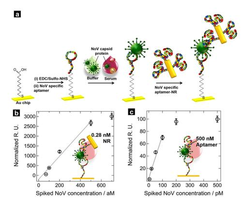
**Figure 5.** (a) Schematic illustration of SPR sensor fabrication via the sandwich aptamer technique. (b) Linear plot of norovirus spike protein-sensing performance. (c) Linear plot of norovirus spike protein-sensing performance without gold nanorods. With permission from [88], Copyright 2018, American Chemical Society.
