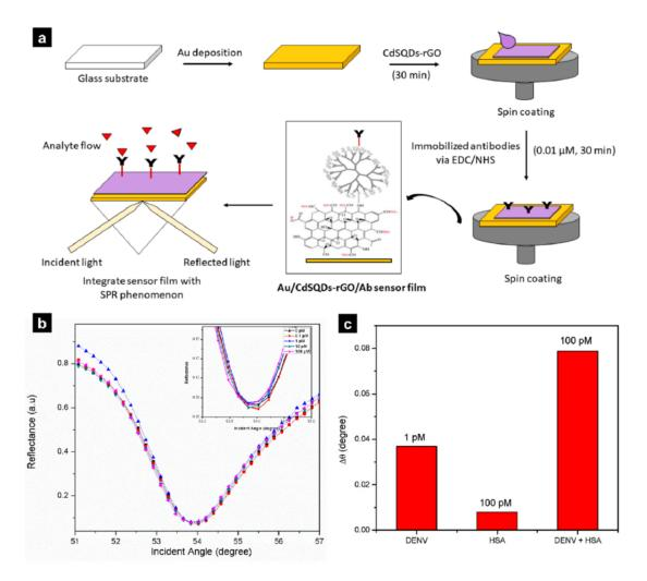
**Figure 4.** (a) Schematic illustration of the biosensor fabrication process. (b) Plot indicating the limit of detection and linear range. (c) Selectivity of the fabricated platform. With permission from [83], Copyright 2019, MDPI.
