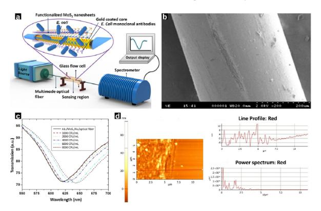
**Figure 6.** (a) Schematic illustration of an experimental setup to test sensors. (b) Field emission scanning electron microscope (FESEM) image of the fabricated optic fibre surface. (c) Transmission spectra plot indicating the limit of detection. (d) Atomic force microscope image analysis of the fabricated optic fibre surface. With permission from [91], Copyright 2018, Elsevier.
