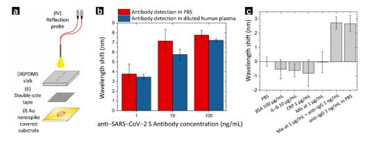
**Figure 3.** (a) Schematic illustration of the fabricated gold nanospike-based SPR sensor. (b) Plot representing the detection limit for the analyte. (c) Selective affinity test against other interference substances. With permission from [81], Copyright 2020, ELSEVIER.
