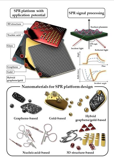
**Figure 1.** Schematic of recent advances in SPR sensor technology with various nanomaterials and applications for pathogen detection.
