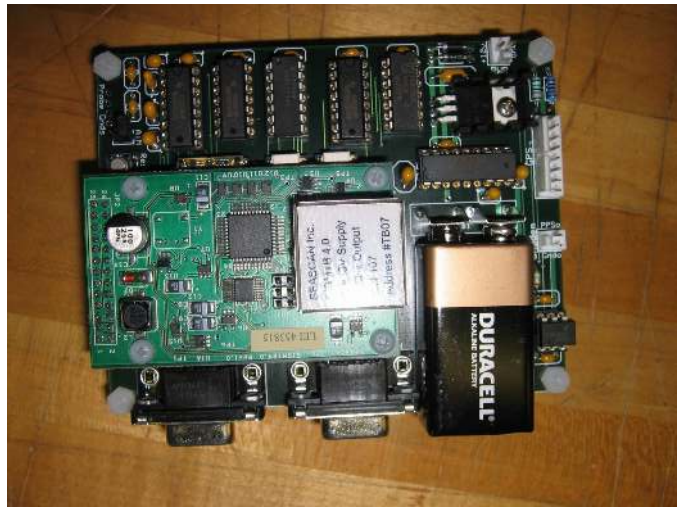
Fig. 1. A depiction of the PPSBOARD designed by the authors. The PPSBOARD integrates a COTS TXCO with a micro-controller based PCB. The PPSBOARD allows for higher-level clock functionality such as PPS synchronization control, measuring of pre and post dive TXCO PPS drift, and generating output suitable for RTC stabilization on the host PC via the open-source NTP algorithm.
