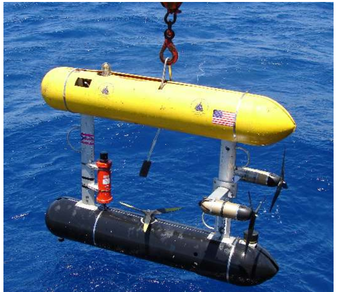
Fig. 3. The SeaBED AUV as used during field experiments. The orange LinkQuest Tracklink beacon mounted on the front strut provided an independent measurement of ship-to-vehicle range.
