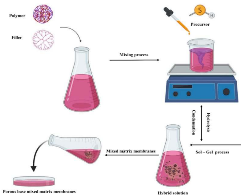
Fig. 10. The Sol-gel steps for constructing a mixed matrix membrane.
