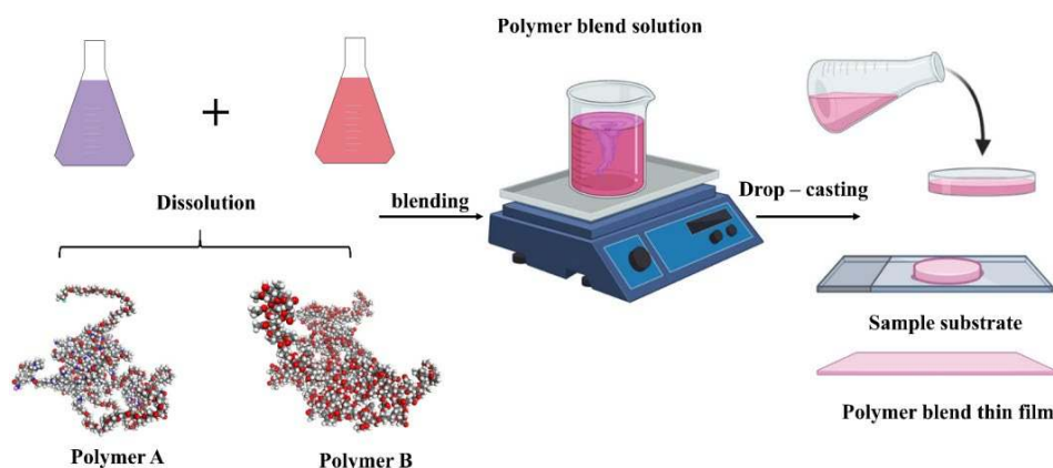
Fig. 4. A general schematic of making a polymer blend using the blending solution method.
