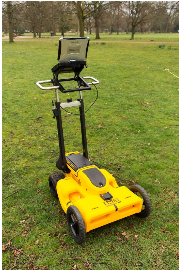
Figure 19: Opera Duo GPR system
