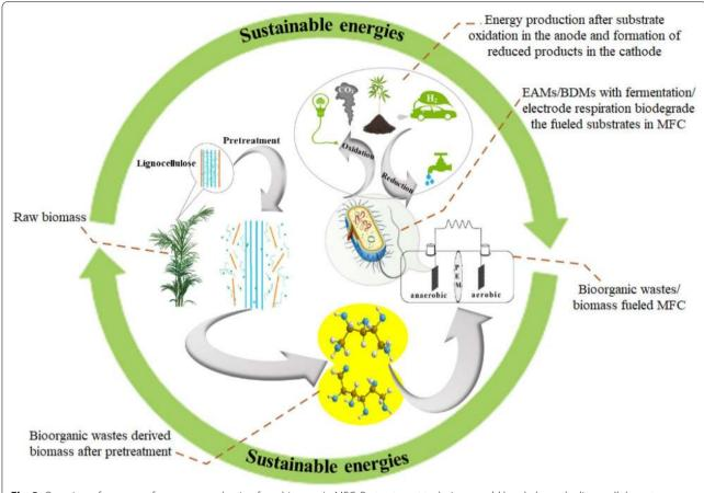
**Fig. 2** Overview of processes for energy production from biomass in MFC. Pretreatment technique could break down the lignocelluloses to reducing sugars, which served the fuels for energy production by EAMs
