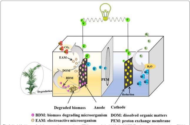
Fig. 1 Model for biomass-fueled proton exchange membrane (PEM) separated microbial fuel cell (MFC). The electroactive microorganisms (EAMs) formed EAMs biofilm and were responsible for the degradation of biomass in the anode
