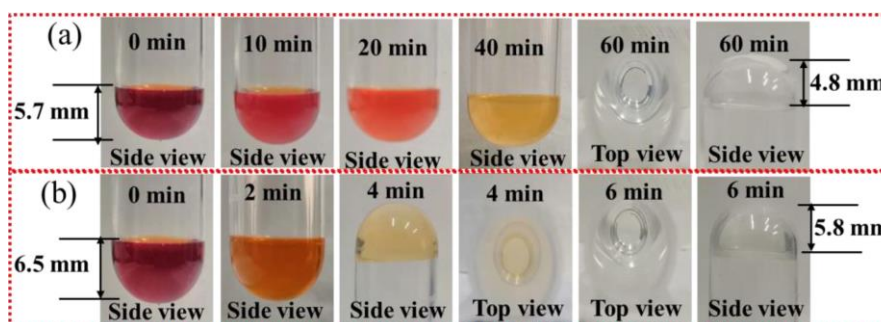
Figure 12. Depth of cure determined during the FRP of HDDA using C10 (a) and TMPTA/EPOX (b) blend using the two-component C10 /Iod2 system upon irradiation at 455 nm. Reproduced with permission of Ref.[141]
