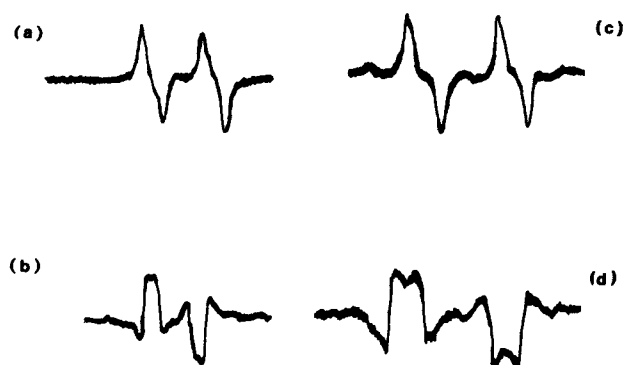
Fig. 6. — Lineshape splitting for high modulation frequencies.
