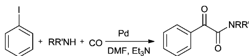
Scheme 78 Reagents and conditions: iodobenzene (0.2 mmol), secondary amine (0.5 mmol), Et 3 N (0.25 mmol), catalyst (3.6 μmol Pd-content), DMF 1 mL, CO 30 bar, temp. 100 °C, time 3 h.
