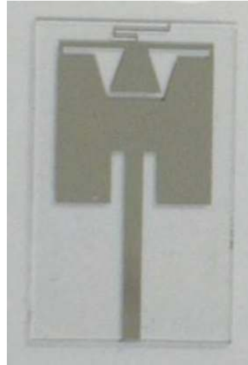
FIGURE 4: Frequency switchable antenna based on MEMS technology [7].
