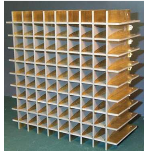
FIGURE 21: Dual-polarized Vivaldi array [45].
