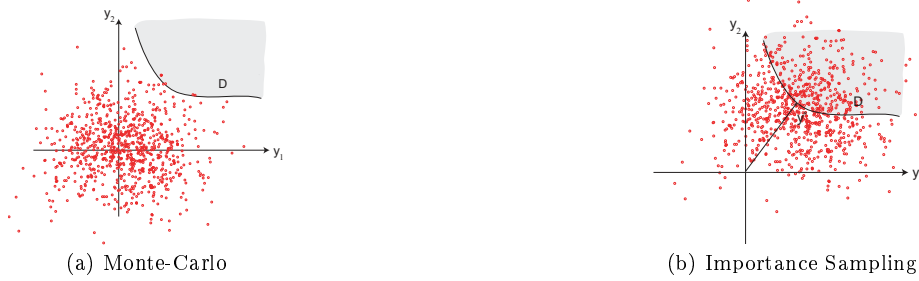
Fig. 6 Simulation methods: standard Monte-Carlo (a), Important Sampling around the conception point \mathbf{y}^*
