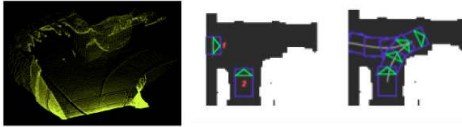
Figure 16. (Left) A 3D point cloud generated at a corridor intersection in the Bruceton Mine. (Center) A binary traversability map of the intersection. Also shown are the robot's initial configuration (1) and its goal configuration (2). (Right) The path planned from the initial configuration to the goal configuration, taking into account steering constraints.
