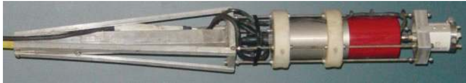
Figure 12. A borehole deployable sonar unit.
