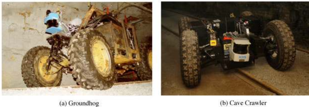
Figure 14. Groundhog and Cave Crawler, our two subterranean mobile robots.
