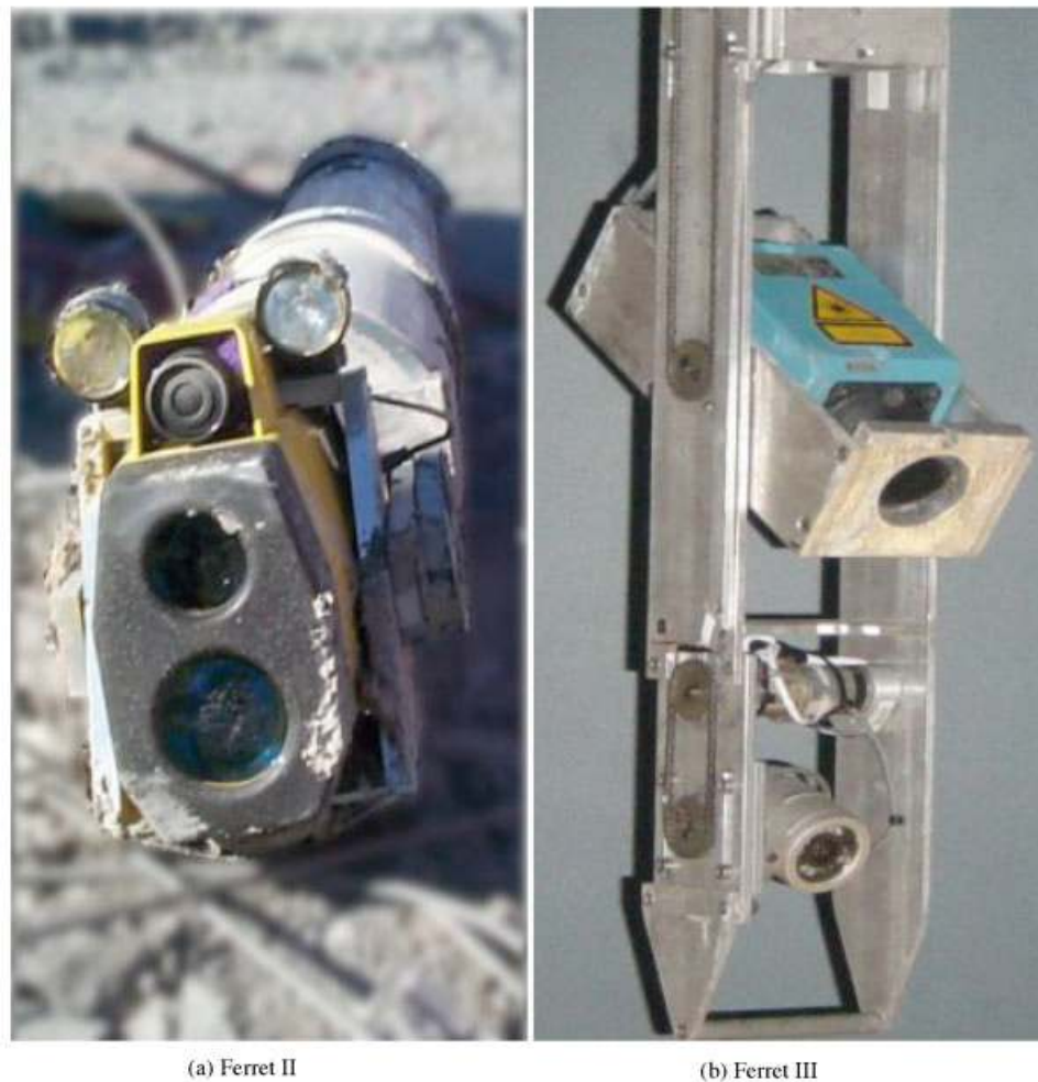
Figure 7. Borehole deployable lasers developed to scan subterranean voids.
