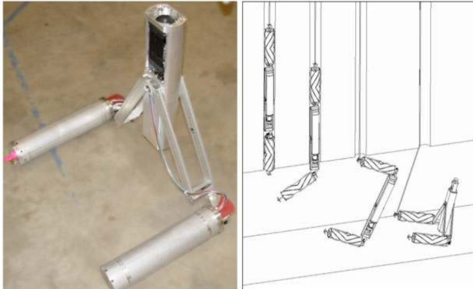
Figure 22. (Left) Photograph of Helix, a mobile subterranean robot that can transform for deployment through boreholes. (Right) A diagram of Helix as it unfolds from a deployment configuration to a mobile configuration.
