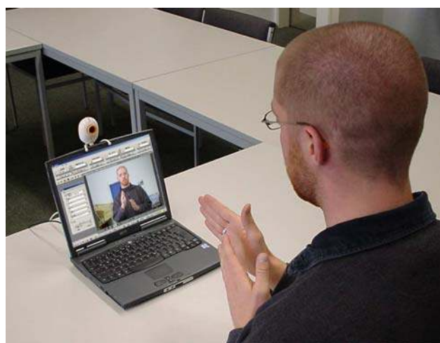
Fig. 1 Laptop and webcam-based sign language recognition system
