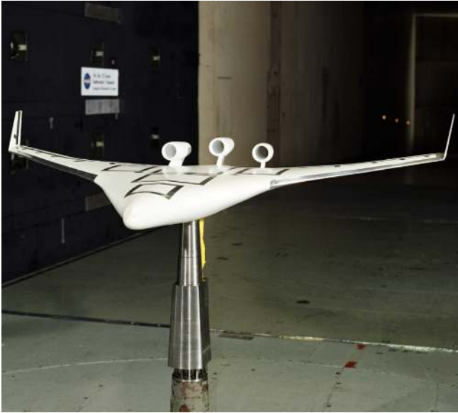
Fig. 5 Blended Wing Body model mounted in NASA-Langley 14- × 22-Foot Subsonic Wind Tunnel.
