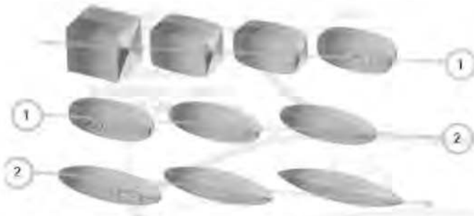
Figure 18. Three variable morphing of a cube into a Sears-Haack body.
