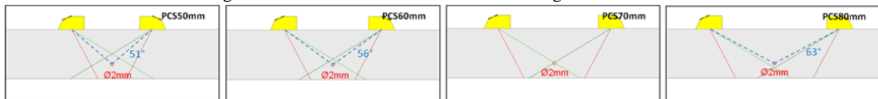
FIGURE 11: SDH at 20mm depth, ray path display and value of the direct ray incidence angle on the SDH. TOFD inspection, contact probe \varnothing 6.35\text{mm} , 5MHz, P60°, various PCS.
