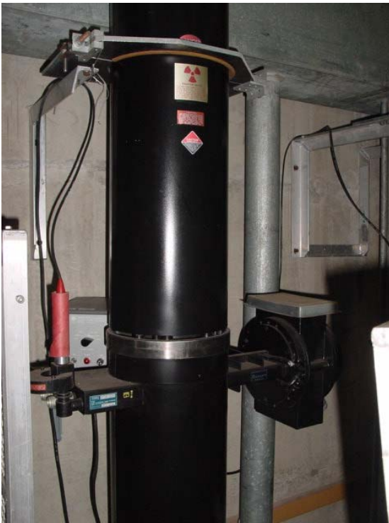
Figure 4: Typical ORELA klystron.
