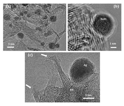
**Figure 4.** Heterogeneous FePt/*h*-BN (a,b) and Ag/*h*-BN (c) catalysts. Arrows show active *h*-BN edges.
