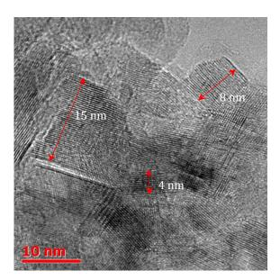
**Figure 3.** Homogeneous BNNSs with an average size of 10 nm synthesized by one-stage low-temperature ammonolysis of boric acid (ammonothermal dehydration method).
