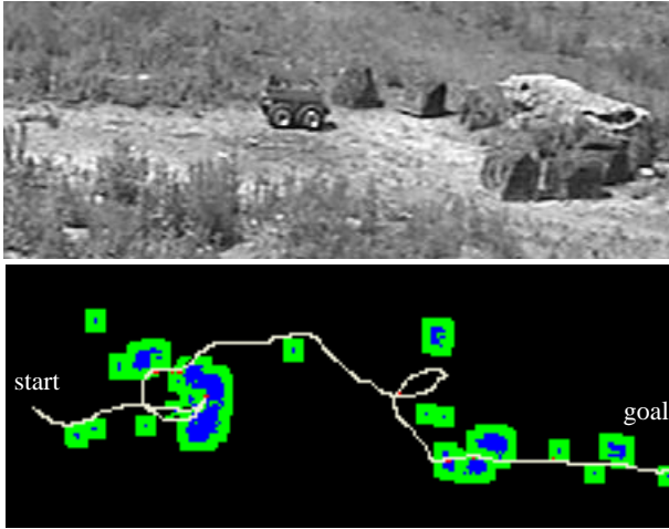
Fig. 7 Results from a field trial (above) Bullwinkle negotiates a cul-de-sac with no prior knowledge of the environment. (below) Final map created by D* after a 60 m traverse.
