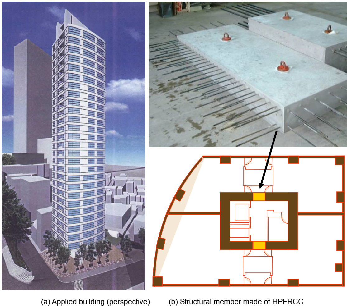
Fig. 12 Outline of damper in building (Maruta et al. 2005).
