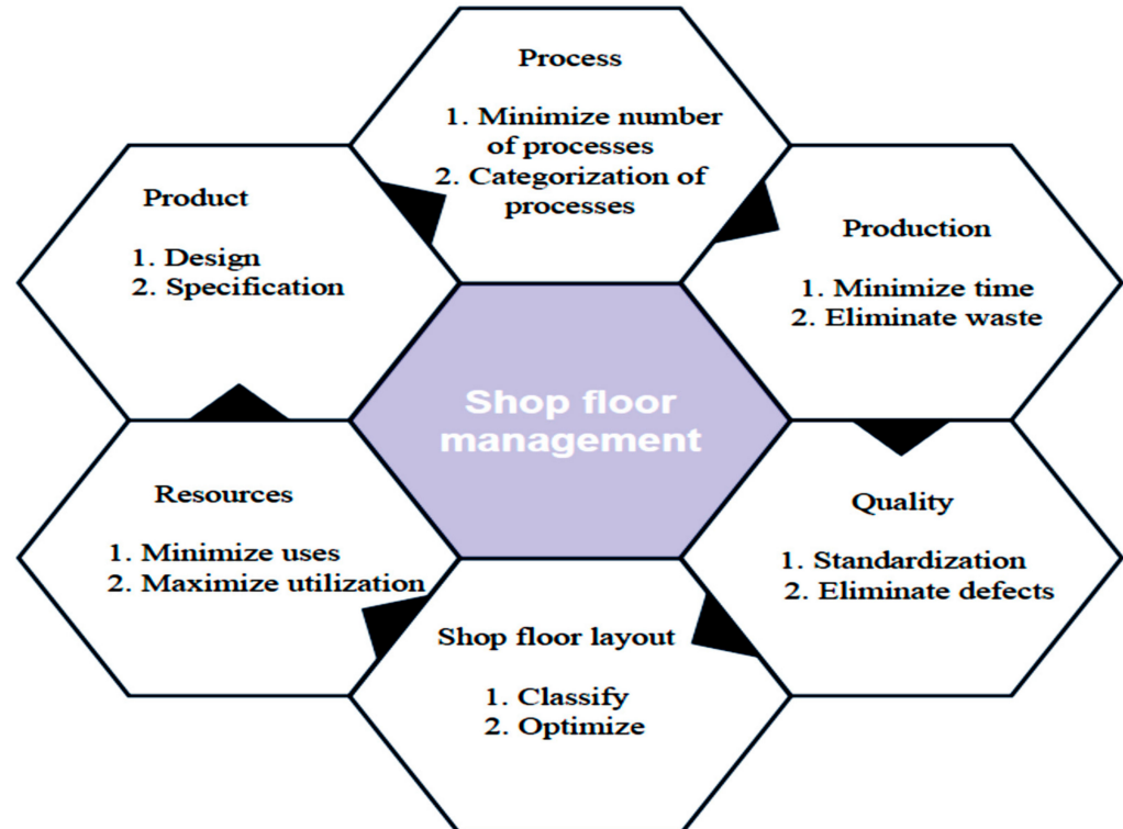
Figure 15. Production parameters for shop floor management.
